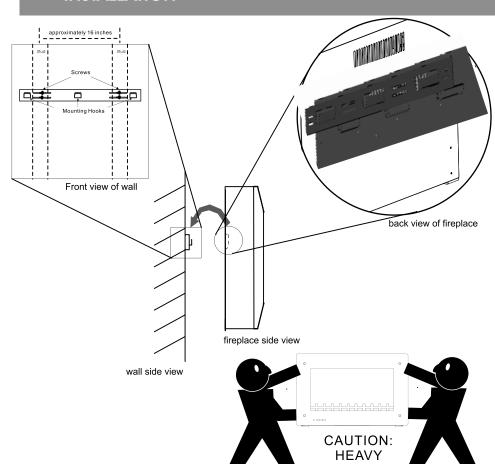
This fireplace must be mounted on a wall with a height above the floor between 0.5M (1.64 Feet) and 2.5M (8.2 Feet).
